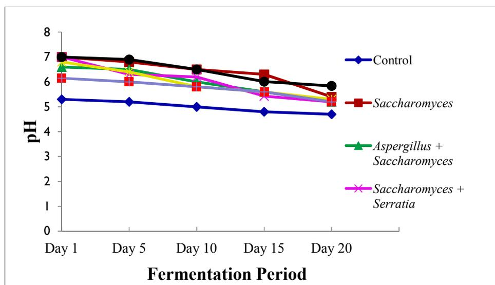
Fig. 4. pH variation during the production of bio-ethanol from the rhizome extract of *Imperata cylindrica*
