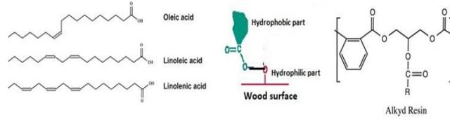
**Fig. 1. Wood surface bonding potentials with fatty acids and alkyd resin**
