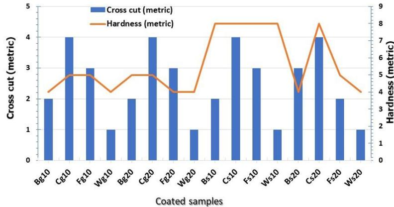
**Fig. 2. Cross cut and hardness changes of wood species**
